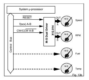
A partial step is an angular rotation of  $1/3^{\circ}$  of the M-S shaft or  $60^{\circ}$  on the rotor shaft.
